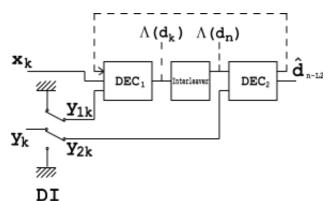
An interleaver installed between the two decoders is used here to scatter error bursts coming from output. DI blocks is a demultiplexing and insertion module, it works as a switch redirecting inputs bits to at one moment and to at another. In OFF state, it feeds both and inputs with padding bits.
